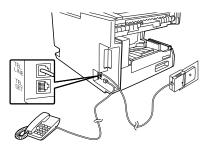
**Important:** In New Zealand, not all standard telephones will respond to incoming ringing when connected to the extension socket of the equipment.
